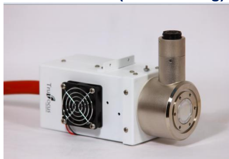
Packaged in a metal housing with FAN
